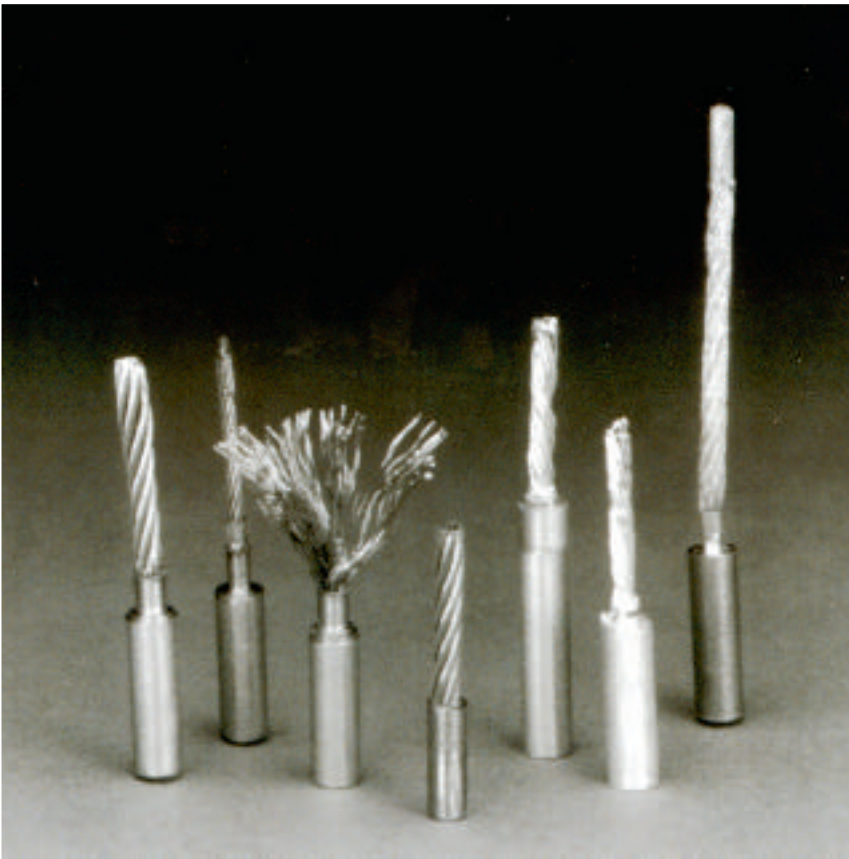
Capacitor discharge welding can be used to join dissimilar metals without fluxes and without the typical problems involving heat-affected zone failures.
