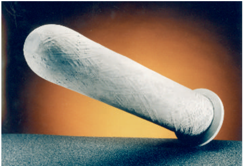
The tube shown here is a sample of continuous fiber ceramic composite (CFCC) made of silicon nitride-bonded silicon carbide in a rapid densification process developed by Textron Specialty Materials with DOE funding. The CFCC tubes are the key components of a new aluminum melting system called an immersion melter.
