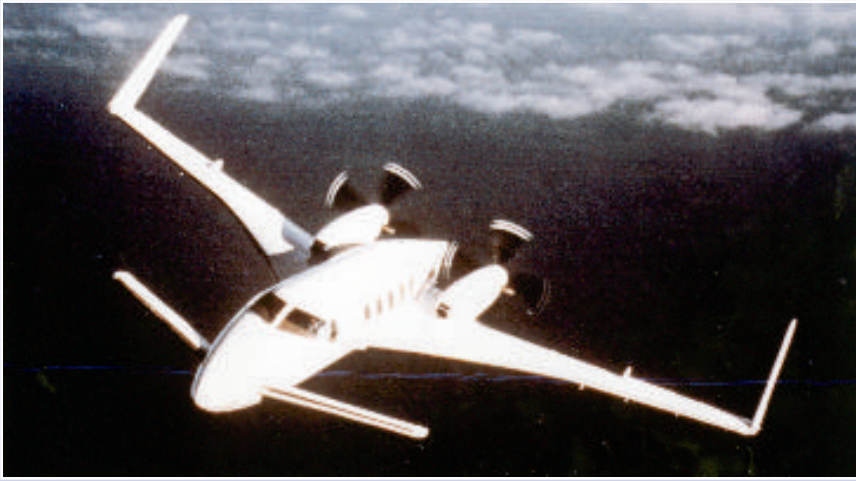
To meet crashworthiness standards and ensure operational safety, the FAA R&D program tests a variety of aircraft types, such as the all-composite Beech Starship aircraft in the photo.
