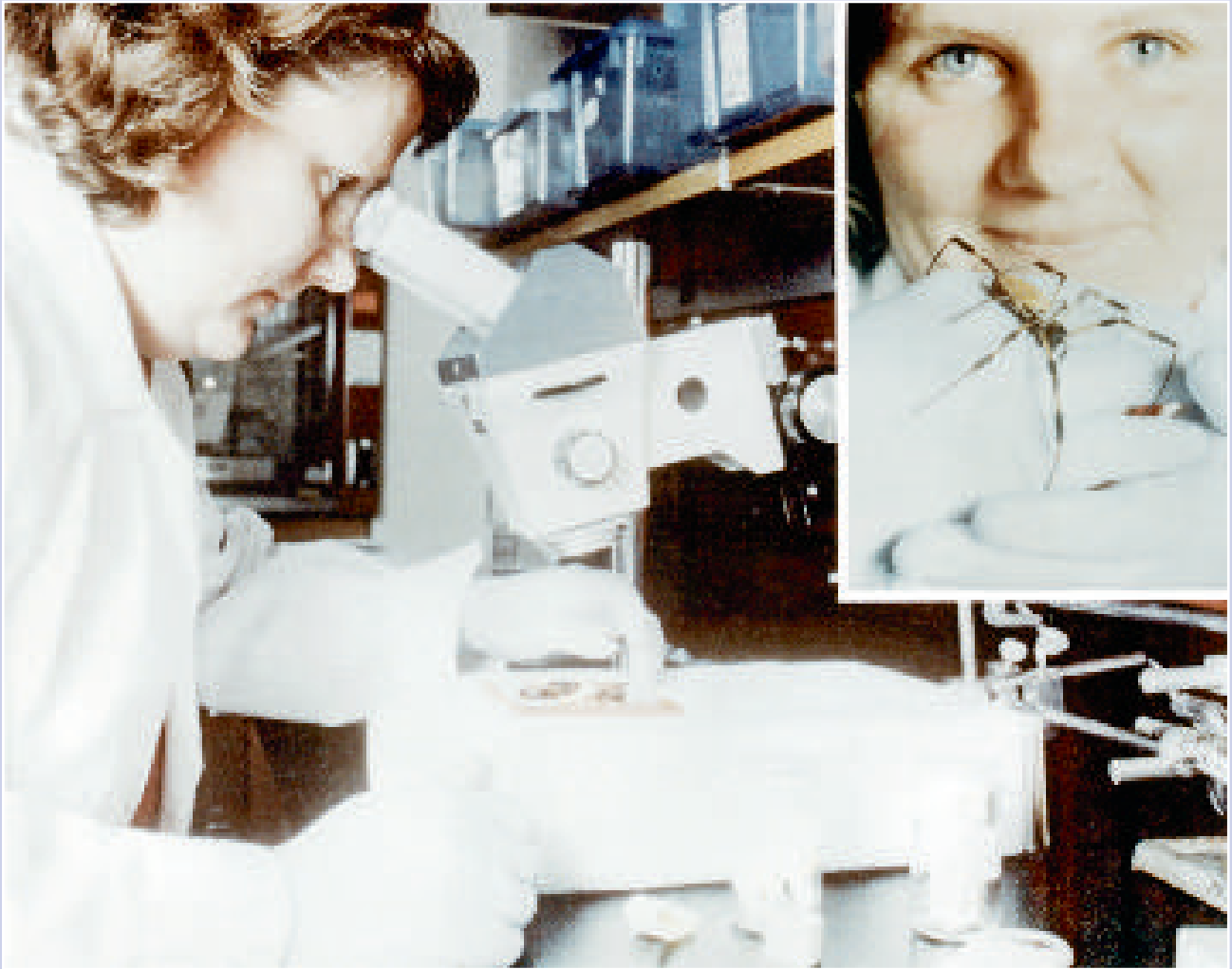
A silking apparatus permits separation of dragline silk from other silks and pulls it onto a rotating white drum. A postdoctoral student from Cornell University is holding one of the golden, orb-weaving spiders that produce the dragline silk.
