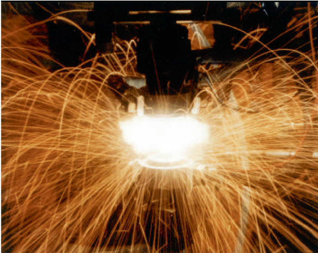
Wire joined to stubs by capacitor discharge welding, which minimizes heat-affected zones and does not require the use of dangerous fluoride-containing fluxes.
