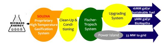
The BTL facilities are designed to process 592,000 metricTons/year of biomass feedstock to produce (i) sixteen million gallons of sustainable aviation or marine fuel; (ii) nine million gallons of sustainable naphtha; and (iii) 33 MW of baseload electricity that are exported/sold to the grid.
