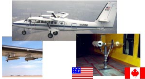
Figure 2: Twin-Otter and Droplet Particle Measuring Probes (on aircraft and in tunnel)
