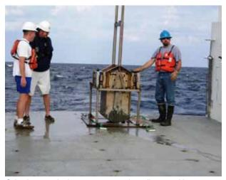
Scientists use the box corer to sample sediments with negligible disturbance. Sediment cores are used to study sediment-oxygen-nutrient dynamics. Photo. L.Jewett, NOAA
