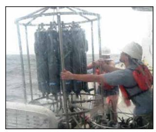
Researchers retrieve the CTD rosette, used for collecting water and measuring dissolved oxygen and other oceanographic parameters, after a sampling profile is completed during rough seas.
