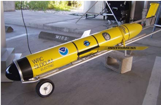
The Slocum Glider AUV with “Brevebuster,” an automated sensor for detecting Karenia brevis . Photo: NOAA
