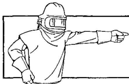
**Fig. 1. Supplied air respirator, hood style, Type CE.**
