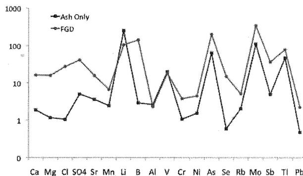
**Figure 2.** Mean values of enrichment factors of dissolved constituents in CCR effluents disposed from plants with an FGD system (red) and without an FGD system (blue). The enrichment factors were calculated by the ratio of different elements concentrations in directly sampled CCR effluents to the concentrations in the upstream water that feeds each plant.
