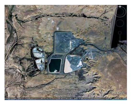
The potential for the ash ponds to pollute the Chaco Wash with a variety of metals concentrated in the ash is clear. Ross (2007) found that concentrations of antimony, arsenic, boron, cadmium, cobalt, copper, iron, manganese, molybdenum, nickel and zinc are significantly higher in samples of ash in the ponds than found in any other source material in the area (in the analysis samples were segregated into 18 categories for comparison).
