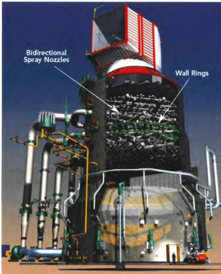
Figure 2-1. Typical Wet FGD Absorber Tower
