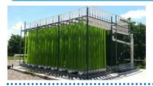
A demonstration scale photobioreactor is currently being operated and expanded at Duke Energy's East Bend Station located in Union, KY. The PBR converts the CO<sub>2</sub> in flue gas to algal biomass, via photosynthesis. The biomass is then periodically harvested to supply feedstock for upgrading into value added products. The low energy harvesting system recycles water and unused nutrients.
