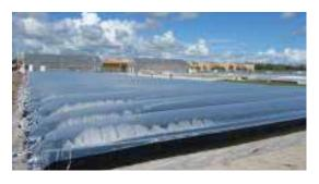
Algenol uses fully closed and sealed photobioreactors for ethanol production directly from enhanced algae. Waste algae are converted into diesel, jet fuel and gasoline using hydrothermal liquefaction and other conversion technologies.
